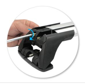
• Tighten adjusting screw to 5 Nm.
